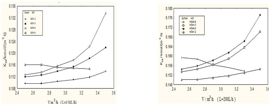
Figure 1: The influence of flow rates and baffle plate spacing  $H/D$  on the  $K_{Xa}$ .
