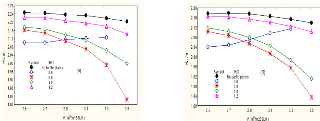
Figure 2: Height of mass transfer unit vs. baffles.
